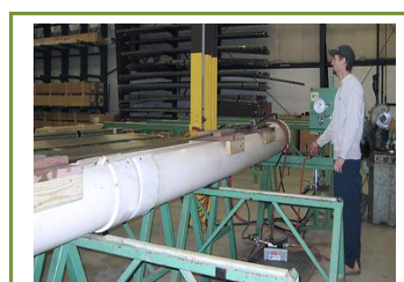
Hydrostatic Pressure Test
