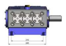
Note: All dimensions are in mm & weight of bare pump is 85 Kg approx.
