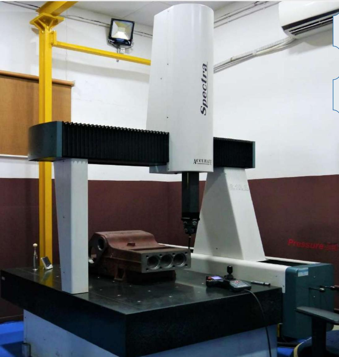
CMM for GD&T measurement of components
