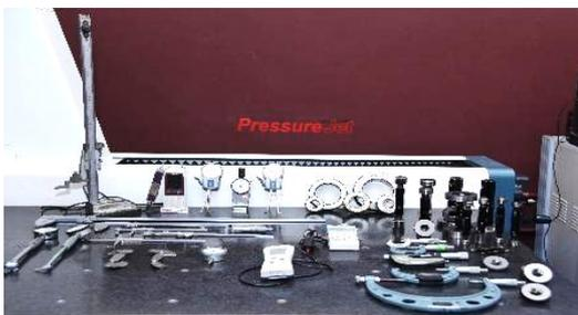
2. Thoroughly check each component of DIFFERENT pumps and accessories, using over 257 quality checking instruments including CMM. No other manufacturer can claim to have such variety of Quality checking instruments, which are essential to ensure technically correct products.
