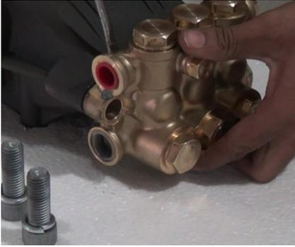
Once separation has been made, use one flat tip screw driver to separate manifold to the crankcase
