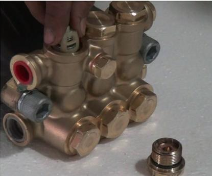
**Install valve assembly into manifold and pressing at the place.**
