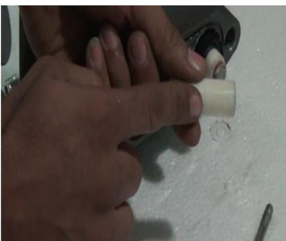
Remove plunger and check for any damage or cracks or cuts.
