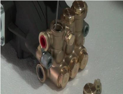
While removing the valve assembly, the O-ring may remaining in the manifold. Using small picker screw driver retain to the manifold to remove, Inspect the O-ring for cuts and nets or any damage.
