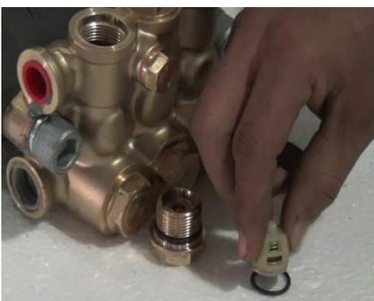
Replace the O-ring and lubricate before installing into the manifold.
