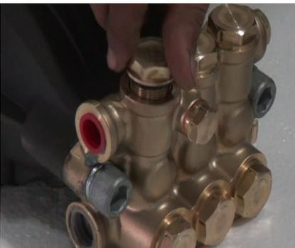
**Lubricate the O-ring and reinstall valve plug.**
