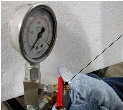
**Needle valve must be open during increase pressure.**
