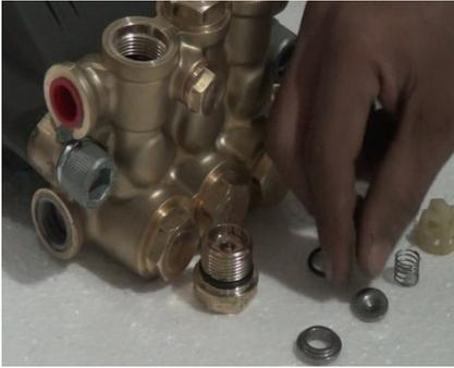
To reassemble the valve assembly
