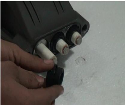
Check seals for any damage or cuts on it.
