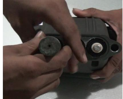
**Install the oil seal. To install the oil seal use proper tool, use plastic hammer to place it completely.**
