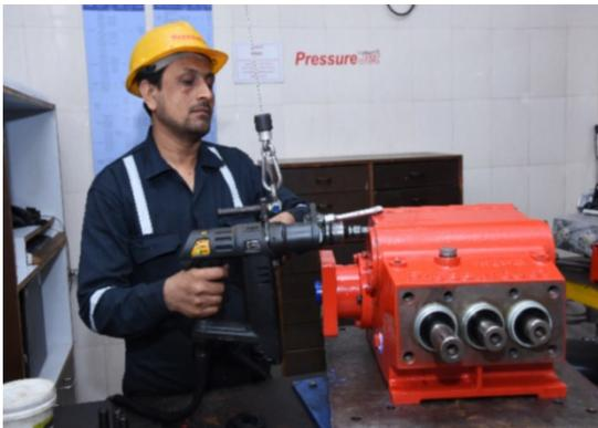
8. Use state-of-the-art Atlas Copco make **electric torque wrench** to tighten all bolts in your pump. Ensures perfect fitting of all parts of your pump. This ensures long life of parts. This is one of the reasons, PressureJet is the only supplier which insists customer to opt for **24 hours continues duty test**, before finalizing the order and committing your major investment. No other High PressureJet Pump manufacturer in the world uses this highly sophisticated, latest tool.
