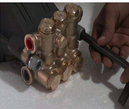
**Use 10 mm LN Key to open the manifold. To service or repair the seals it is compulsory to open the manifold.**
