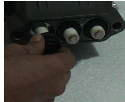
**To install the seal of power end on plunger, first of all place the O-ring on seal.**
