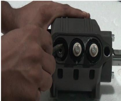
**Remove Oil seal after removal of copper spacer.**
