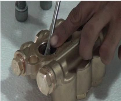
To check, service or replace the seal, Use flat tip screw driver and gently remove the seal.
