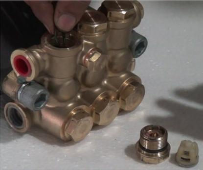
**Install the O-ring into the manifold.**
