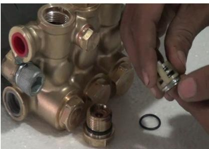
And then place spring retainer on spring and press to assemble whole assembly.
