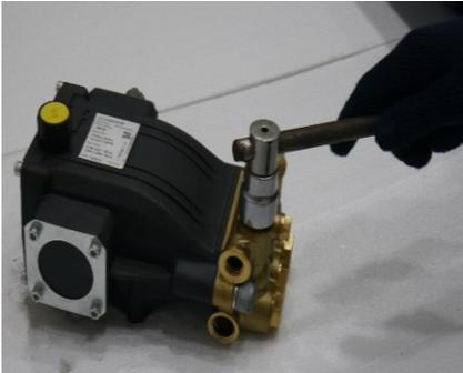
**To remove the valve plug, using the 24 mm hex wrench.**
