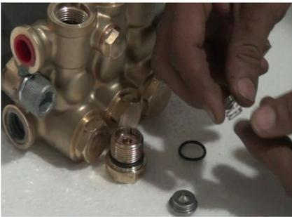
Place valve on the valve seat with taper surface of valve facing down.
