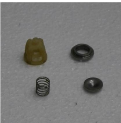
Inspect spring retainer for cracks, excusable wear or damage.
