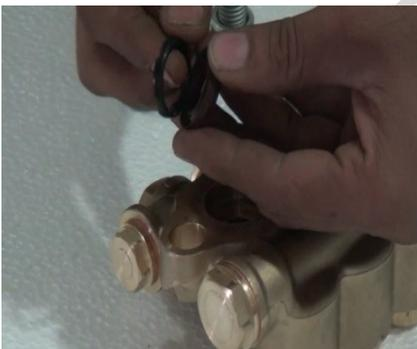
Separate the seal and low pressure seal and check for any damage or cuts on that.
