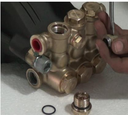
If the valves is going to be reused, serviced or inspected, the assembly can be dismantled.
