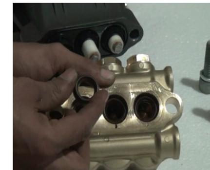
To install the seal in manifold. Install low pressure seal first into a hole of manifold.
