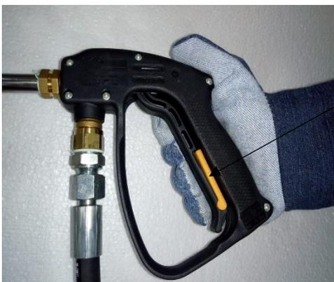
**Press Trigger Gun during increase Pressure using PRV or Unloader Valve.**
