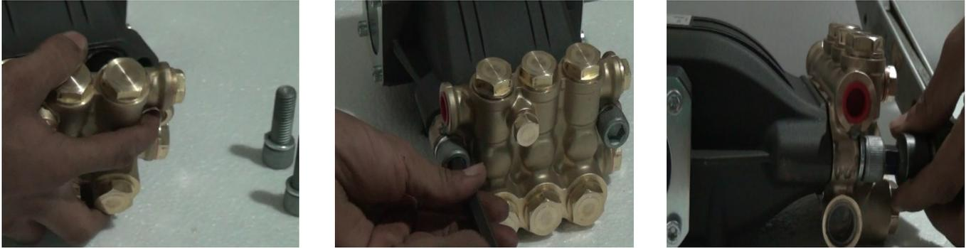
Then install a manifold and tighten it through their bolts.
