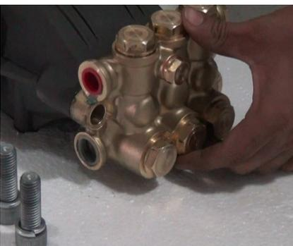
**To create separation between the manifold and crankcase, rotate the crankshaft and there is a gap between the manifold and crankcase.**
