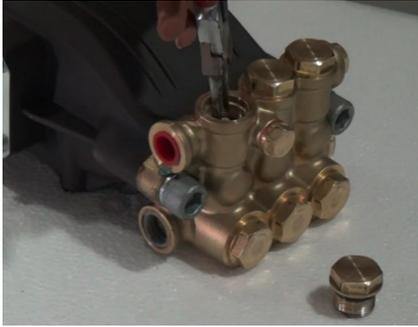
To remove the valve assembly, Use needle nose pliers grasping the top of the spring retainer, pull the valve outside.
