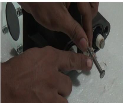
Remove whole screw from the plunger with copper washer.
