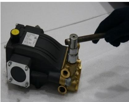
**After removing the valve plug inspect the O-ring for cuts or any damage. (New O-ring is included with the valve kit.)**
