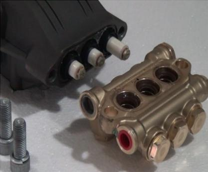
After the separation, place manifold on flat surface with seals facing up.
